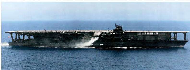
HIJMS Kaga was originally laid down in 1920 as a battleship of 39,900 tons, HIJMS Kaga was converted into an aircraft carrier as the result of the Washington Treaty. Smoke is discharged through huge trunks on both sides, extending for nearly half the length of the ship and turning outboard towards the stern. There is accommodation for 60 planes.
